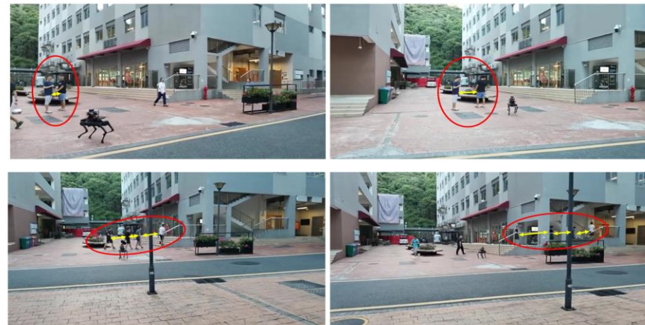
Fig. 9: Examples from the real-world experiment. The top and bottom images describes two different scenarios. Left: The robot detected and approached the crowds, then persuaded them to keep social distance. Right: The crowds density decreased.
